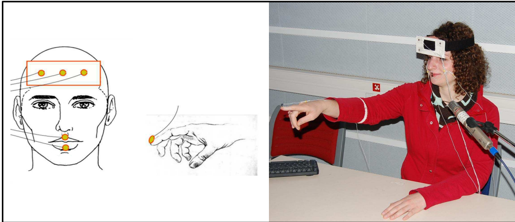
FIGURE 3.2 – Position des diodes émettrices infra-rouge (© C. Gonseth)
