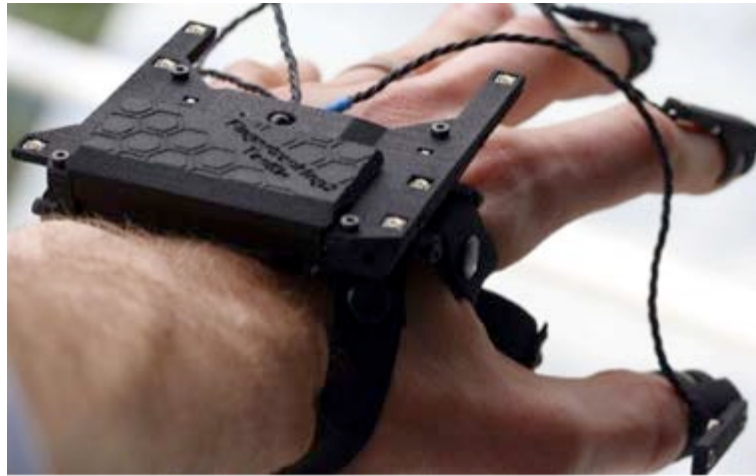
Figure 5.3: ART finger-tracking system (from https://ar-tracking.com/ )
