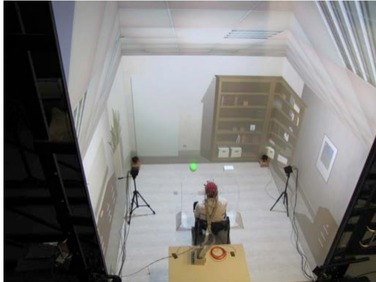
Figure 5.2: Cave automatic virtual environment (CAVE). The virtual environment represents an office, with a desk on which the participant can manipulate objects.
